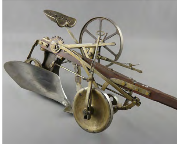
Contemporary photo of John Groat's Sulky Plow, a horse-drawn plough with a seat. This heavy iron plough had a lever to control the depth of the blade. This model one numerous awards (see below) (Grimsby Museum Collection).
