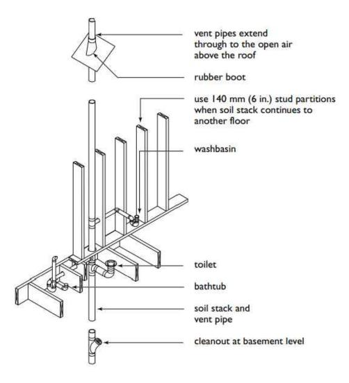
In partitions, holes may be drilled in studs if the remaining portion totals at least 40 mm (1½ in.); otherwise studs must be suitably reinforced.
