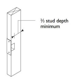
In load-bearing walls, notched studs need not be reinforced if remaining portion is at least  $\frac{2}{3}$  the depth of the studs.
