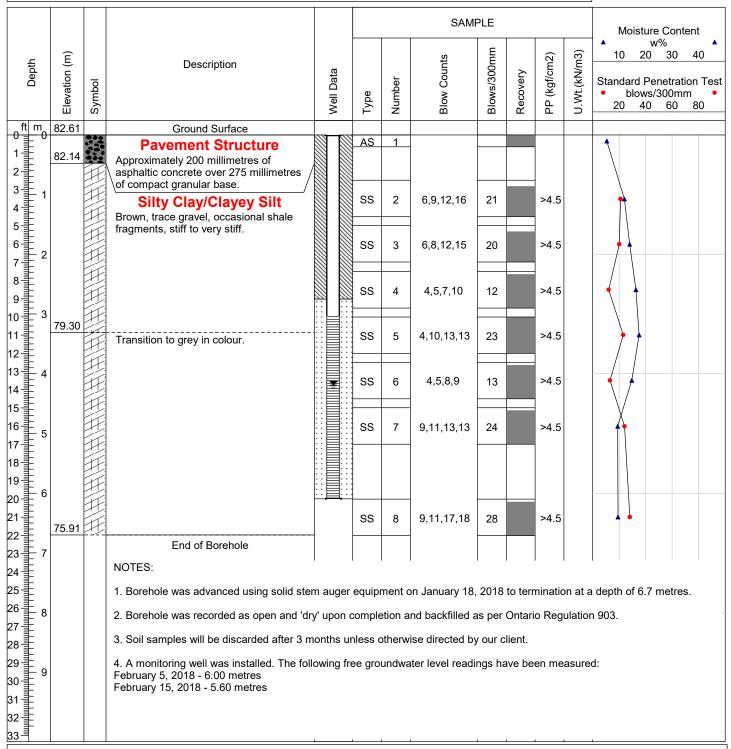
Drill Method: Solid Stem Augers Drill Date: January 18, 2018 Hole Size: 150 millimetres **Drilling Contractor:** Elite Drilling
