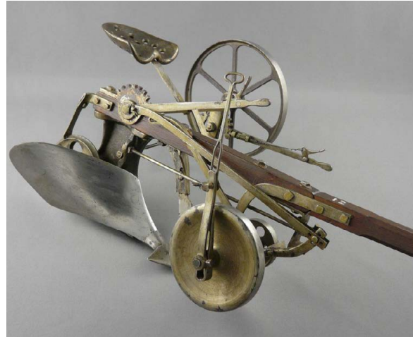
Contemporary photo of John Gout's Sulky Plow, a horse-drawn plough with a seat. This heavy iron plough had a lever to control the depth of the blade. This model one numerous awards (see below) (Grimsby Museum Collection).
